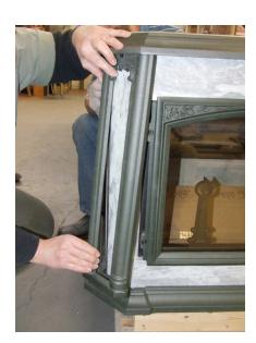
3. The tie rods are fastened with a ½" hex nut, which is located close to the leg bolts. Loosen the tie rod by loosening the nut. About 4 full revolutions. Now lift upward on the large top frame just above the first of the cast corners and remove the cast corner as previously described. Repeat this process for the other front cast corner.
